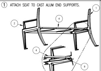
2 ATTACH BACKREST TO CAST ALUM END SUPPORTS. ATTACH BACKREST TO SEAT AT FOUR TAPPED LOCATIONS.
