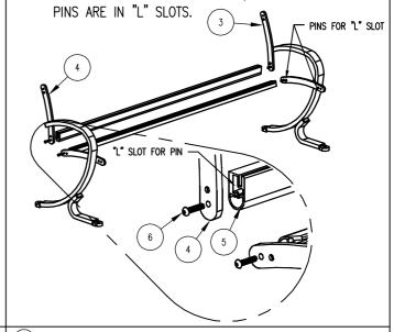
$(\mathbf{3})$  insert step 1 into step 2, USING SLOTS ON ALUM. EXTRUSION.
