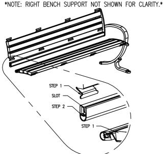
(4) ATTACH 2 REMAINING ALUM. EXTRUSIONS TO SUPPORTS, AS IN STEP 2.
