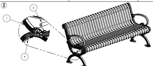
ATTACH 71 3/4" PIPE BRACE TO STEP 1 ASSEMBLY
