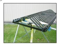
PLACE SEAT ASSEMBLY ON WORK SURFACE ALLOWING ACCESS TO ENDS. PLACE RATCHET STRAP AROUND SEAT ASSEMBLY AS SHOWN ABOVE.
