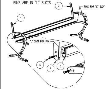
(3) INSERT STEP 1 INTO STEP 2, USING SLOTS ON ALUM. EXTRUSION.
