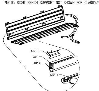
4 ATTACH 2 REMAINING ALUM. EXTRUSIONS TO SUPPORTS, AS IN STEP 2.
