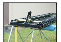
PLACE SEAT ASSEMBLY ON WORK SURFACE ALLOWING ACCESS TO ENDS. PLACE RATCHET STRAP AROUND SEAT ASSEMBLY AS SHOWN ABOVE.
